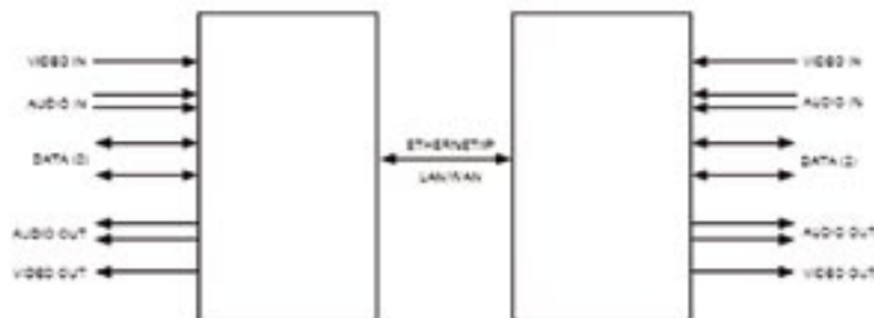
DUPLEX ETHERNET/IP VIDEO/AUDIO COMMUNICATIONS LINK
